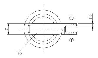
Tab material : Plated stainless steel with Pb free Tab thickness : 0.15mm Welding strength of tab : Min.19.6N (Vertical direction from welding plate)
