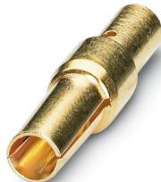
Crimp contact, Socket, turned, contact diameter: 1 mm, crimp range: 0.14 mm<sup>2</sup> ... 0.56 mm<sup>2</sup>,
