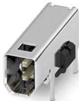
SPE PCB connector, design: IEC 63171-2, degree of protection: IP20, number of positions: 2, 1 Gbps, CAT B (ISO/IEC 63171), material: Metal, connection method: THR solder connection, cable outlet: straight, Single Pair Ethernet
