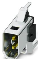
SPE PCB connector, design: IEC 63171-2, degree of protection: IP20, number of positions: 2, 1 Gbps, CAT B (ISO/IEC 63171), material: Metal, connection method: THR solder connection, cable outlet: straight, Single Pair Ethernet
