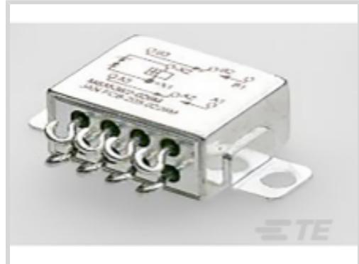
Relay & Contactor Type: **General Purpose Power Relay**Current Type: **DC**Coil Magnetic System: **Polarized, Monostable**Contact Arrangement: **2 Form C DPDT-CO**Contact Current Rating: **5 A**
