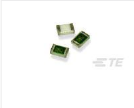
TE Part #4-1879208-1 CPF 0402 470R 0.1% 25PPM 1K RL
