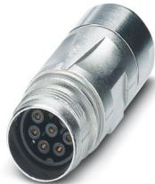
Coupler connector, straight, for standard and SPEEDCON interlock, M17, number of positions: 5+3+PE, contact connection type: Socket, shielded: yes, degree of protection: IP67, cable diameter range: 3.5 mm ... 5.5 mm, number of positions: 9, connection method: Crimp connection, series: ST, Alternative product in accordance with RoHS II without Exemption 6c (Pb < 0.1 %) item no.: 1243307
