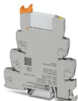
PLC-INTERFACE, consisting of basic terminal block PLC-BSC.../21 with screw connection and plug-in miniature relay with power contact, for assembly on DIN rail NS 35/7,5, 1 changeover contact, input voltage 125 V DC
