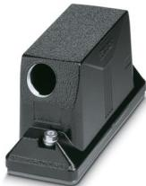
Sleeve housing B24, with screw locking, material: Die-cast aluminum, salt water resistant, cable outlets: 1, lateral, 1x M25, height: 74 mm, cable gland: none, increased environmental requirements
