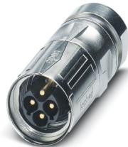
Cable connector, straight, SPEEDCON, M17, number of positions: 5+3+PE, contact connection type: Pin, shielded: yes, degree of protection: IP67, cable diameter range: 10 mm ... 12.5 mm, number of positions: 9, connection method: Crimp connection, series: ST, Alternative product in accordance with RoHS II without Exemption 6c (Pb < 0.1 %) item no.: 1245245
