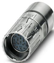
M23, Cable connector, series: M23 PRO, straight, shielded: yes, ONECLICK fast locking system, No. of pos.: 17, Direction of rotation: Standard, contact connection type: Socket, Crimp connection, cable diameter range: 3 mm ... 15 mm, coding: N, Item is lead-free in accordance with RoHS II without Exemption 6c (Pb < 0.1 %)
