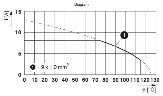
I = current strength,  $\vartheta$  = ambient temperature, 9x 8 A
