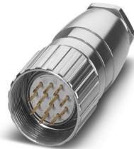
M23, Cable connector, series: RC, straight, shielded: no, Screw locking mechanism, No. of pos.: 17, Direction of rotation: Standard, contact connection type: Pin, Solder cup, coding: N, Alternative product in accordance with RoHS II without Exemption 6c (Pb < 0.1 %) item no.: 1241306
