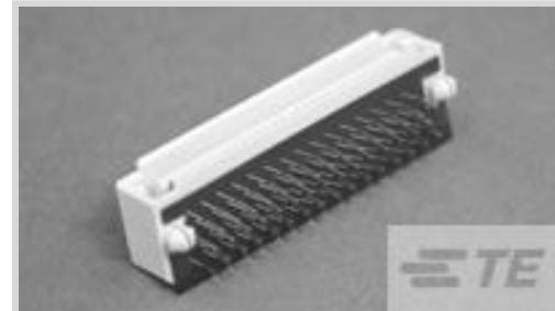
PCB Connector Assembly Type: **PCB Mount Header**PCB Mount Orientation: **Right Angle**Connector System: **Board-to-Board**Number of Positions: **80**Centerline (Pitch): **.8 mm [.031 in]****Features****Electrical Characteristics**
