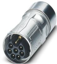
Cable connector, straight, SPEEDCON, M17, number of positions: 7+PE, contact connection type: Pin, shielded: yes, degree of protection: IP67, cable diameter range: 3.5 mm ... 5.5 mm, number of positions: 8, connection method: Crimp connection, series: ST, Alternative product in accordance with RoHS II without Exemption 6c (Pb < 0.1 %) item no.: 1243258
