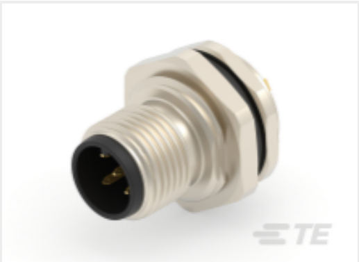
TE Part #T4130012051-000 M12,REAR MOUNT,MALE,A,5P, SOLDER WIRE
