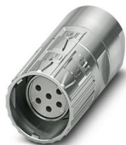
M23, Cable connector, series: M23 PRO, straight, shielded: yes, ONECLICK fast locking system, No. of pos.: 6, Direction of rotation: Standard, contact connection type: Socket, Crimp connection, cable diameter range: 3 mm ... 15 mm, coding: N, Item is lead-free in accordance with RoHS II without Exemption 6c (Pb < 0.1 %)
