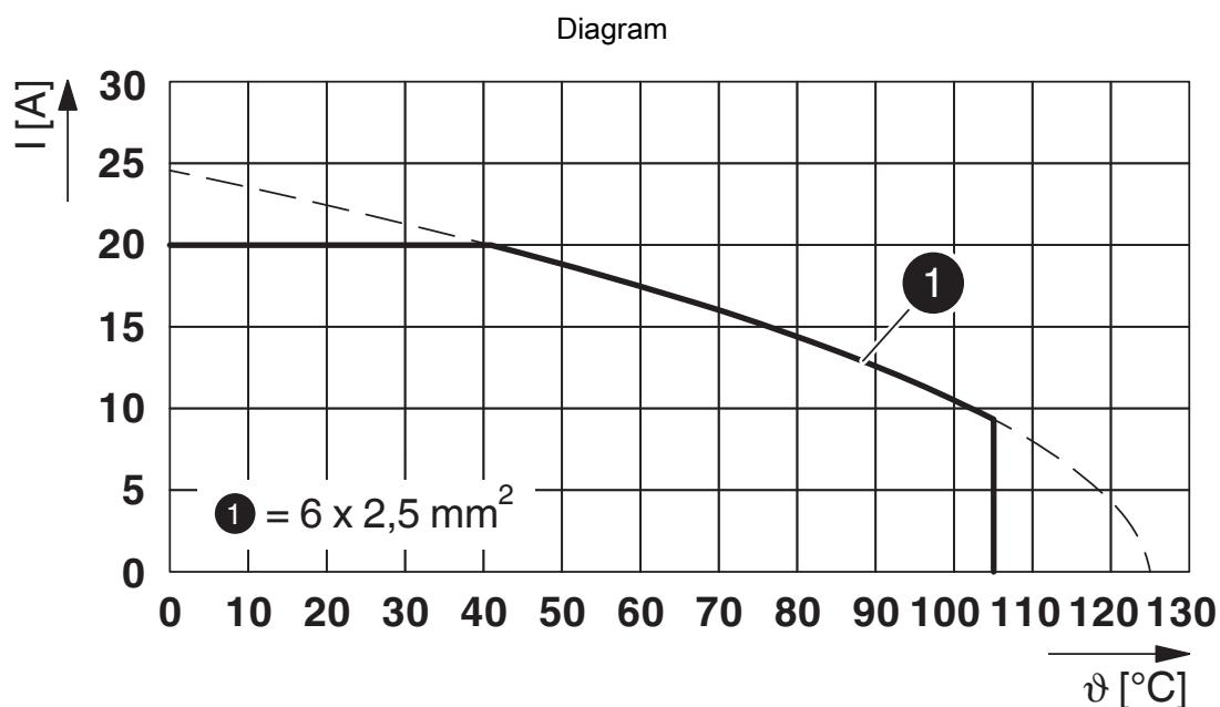
$I$  = current strength,  $\vartheta$  = ambient temperature, 6x 20 A
