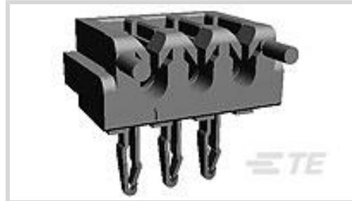
PCB Connector Assembly Type: **PCB Mount One-Piece IDC Connector**PCB Mount Orientation: **Horizontal**Connector System: **Wire-to-Board**Number of Positions: **14**Centerline (Pitch): **2 mm [.079 in]****Features****Electrical Characteristics**
