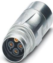
Coupler connector, straight, for standard and SPEEDCON interlock, M17, number of positions: 6+PE, contact connection type: Socket, shielded: yes, degree of protection: IP67, cable diameter range: 5 mm ... 9.2 mm, number of positions: 7, connection method: Crimp connection, series: ST, Alternative product in accordance with RoHS II without Exemption 6c (Pb < 0.1 %) item no.: 1243293
