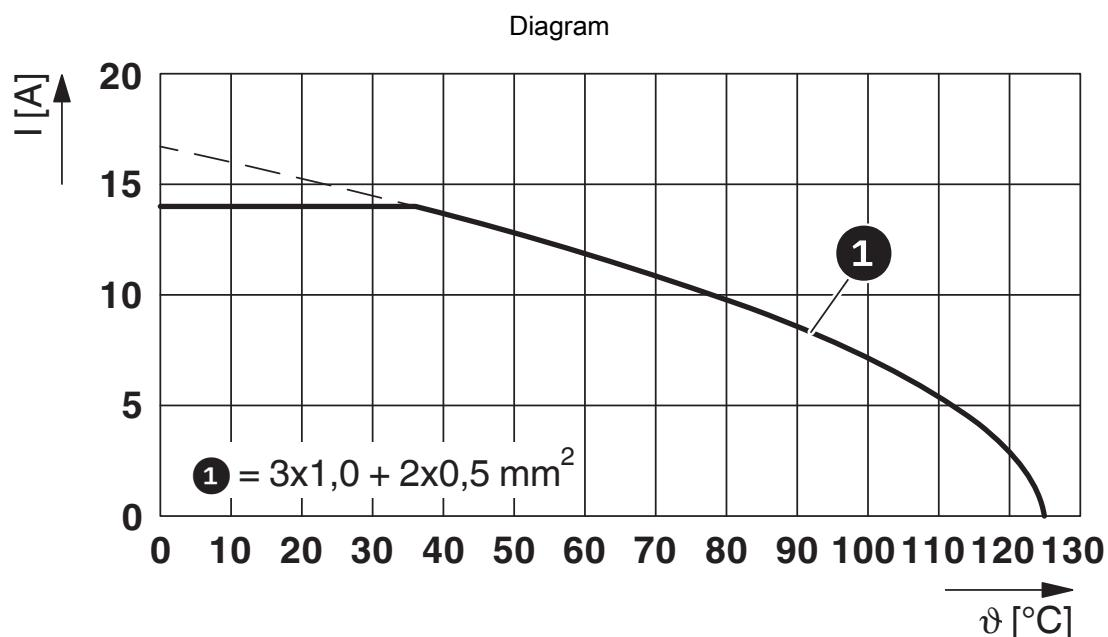
$I$  = current strength,  $\vartheta$  = ambient temperature,  $3 \times 14 \text{ A} + 2 \times 2 \text{ A}$  constant
