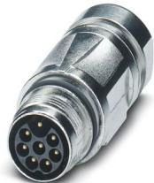
Coupler connector, straight, for standard and SPEEDCON interlock, M17, number of positions: 7+PE, contact connection type: Pin, shielded: yes, degree of protection: IP67, cable diameter range: 10 mm ... 12.5 mm, number of positions: 8, connection method: Crimp connection, series: ST, Alternative product in accordance with RoHS II without Exemption 6c (Pb < 0.1 %) item no.: 1245240
