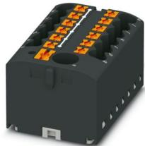
Distribution block, Basic terminal block with supply, nom. voltage: 450 V, nominal current: 24 A, number of connections: 13, connection method: Push-in connection, Load contact, cross section: 0.14 mm<sup>2</sup> - 4 mm<sup>2</sup>, Push-in connection, Line contact, Rated cross section: 6 mm<sup>2</sup>, cross section: 0.5 mm<sup>2</sup> - 10 mm<sup>2</sup>, mounting type: for snapping onto a DIN rail adapter, Direct mounting with flange, Free-hanging, color: black
