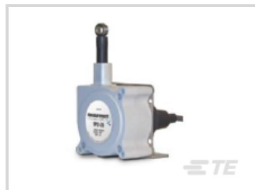
Position Sensor Product Type: **SP Series, String Pots**Full Stroke Range: **101.6 – 1270 mm [4 – 50 in]**Output Signal Type: **Voltage Divider (Potentiometric)**Accuracy: **±.25 % of FS**Repeatability: **.02 % of FS**[All IP67 String Pot, 40in. Electrical Cable \(4\)](#)
