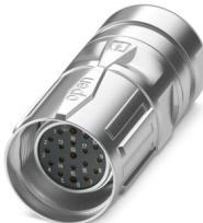
M23, Cable connector, series: CA, straight, shielded: yes, SPEEDCON, No. of pos.: 16+2+FE, Direction of rotation: Standard, contact connection type: Socket, Crimp connection, cable diameter range: 10 mm ... 14.5 mm, coding: N, Alternative product in accordance with RoHS II without Exemption 6c (Pb < 0.1 %) item no.: 1244994
