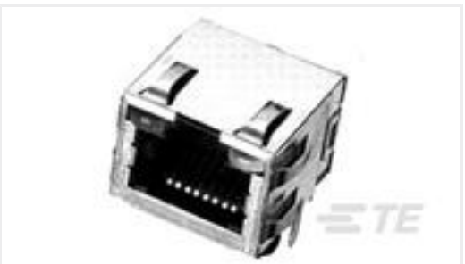
TE Part #6116075-1 INV MJ,1X1,SHIELDED,LED (G/Y)
