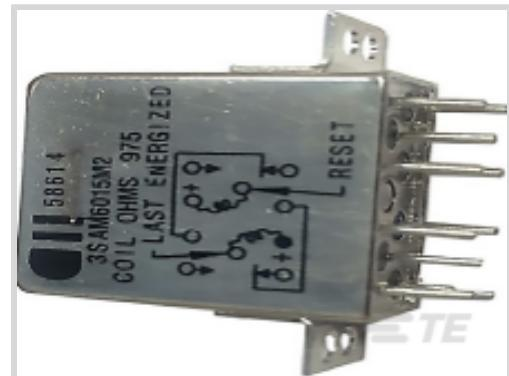
Relay & Contactor Type: **General Purpose Signal Relay**Current Type: **DC**Coil Magnetic System: **Polarized, Bistable, Latching**Contact Arrangement: **2 Form C DPDT-CO**Contact Current Rating: **2 A**[All DPDT Signal Relay: Magnetic-Latched, Full-Size, 2 Form C \(11\)](#)
