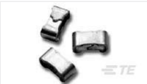
TE Part #1625854-4 1206 PROBE PAD
