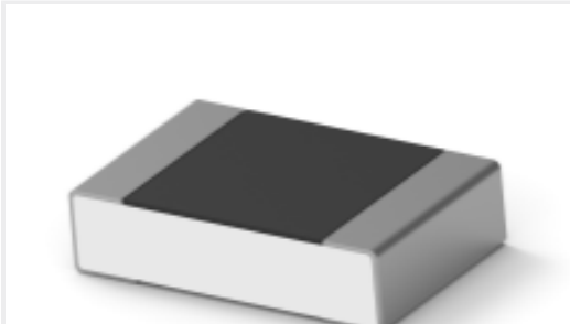
TE Part #3-2176378-4 RQ 0805 22R1 0.1% 10PPM 5K RL
