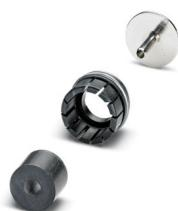
Cable clamp type cage and shield adapter, shielded: yes, litz wire bundle diameter: 5.5 mm, cable diameter range: 5.5 mm ... 6.5 mm, series: NC, RC, Alternative product in accordance with RoHS II without Exemption 6c (Pb < 0.1 %) item no.: 1241803
