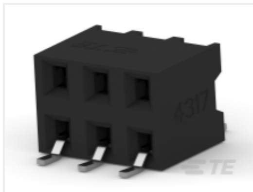
TE Part # 2307730-6 6P,2MM,B-B,REC,DRHZ,SMD,0.38AU, TR
