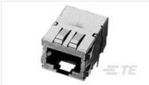
TE Part #1734509-4 RJ45,8P8C,W/LED,G/Y,50u"
