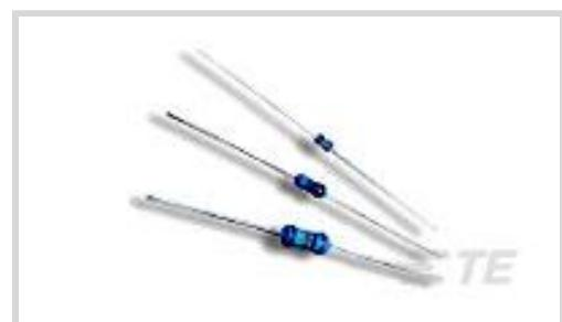
Resistor Type: **Precision Resistor**Element Type: **Thin Film**Power Rating: **.25 W**Resistance Class: **Up to 1kΩ**Resistance Value: **931 Ω**
