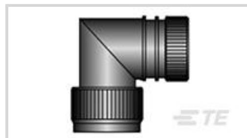
Connector Backshell Product Style: **Screened**Connector Backshell Product Type: **Backshell**Primary Product Material: **Aluminum Alloy**Body Orientation: **Right Angle**Compatible With Connector Shell Size: **09**
