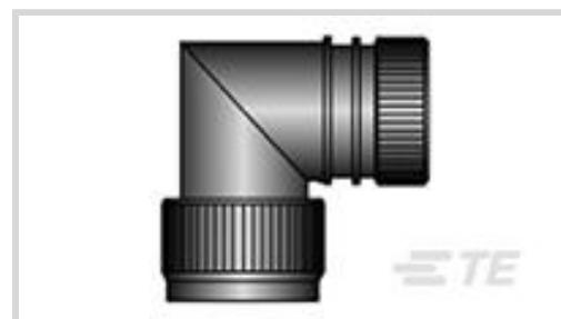
Connector Backshell Product Style: **Screened**Connector Backshell Product Type: **Backshell**Primary Product Material: **Aluminum Alloy**Body Orientation: **Right Angle**Compatible With Connector Shell Size: **09**
