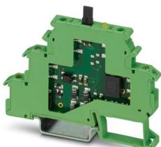
Input solid-state relay terminal block, input: 24 V DC, output: 3 - 48 V DC/100 mA, with isolating plug in output, terminal block width: 6.2 mm
