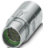
M23, Coupler connector, series: M23 PRO, straight, shielded: yes, for standard and ONECLICK fast locking system, No. of pos.: 12, Direction of rotation: Standard, contact connection type: Pin, Crimp connection, cable diameter range: 9 mm ... 15 mm, coding: N, Item is lead-free in accordance with RoHS II without Exemption 6c (Pb < 0.1 %)
