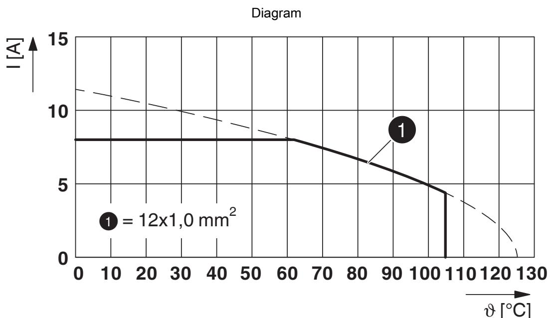
$I$  = current strength,  $\vartheta$  = ambient temperature, 12x 8 A
