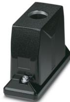
Sleeve housing B24, with screw locking, material: Die-cast aluminum, salt water resistant, cable outlets: 1, straight, 1x M32, height: 93.7 mm, cable gland: none, increased environmental requirements
