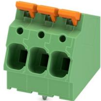
Printed circuit board terminal, nominal current: 41 A, rated voltage (III/2): 1000 V, nominal cross section: 6 mm<sup>2</sup>, number of potentials: 3, number of rows: 1, number of positions per row: 3, product range: LPTA 6/, pitch: 7.5 mm, connection method: Lever Push-in connection, mounting: Wave soldering, conductor/PCB connection direction: 30 °, color: green, Pin layout: Zigzag pinning W, Solder pin [P]: 3.6 mm, type of packaging: packed in cardboard
