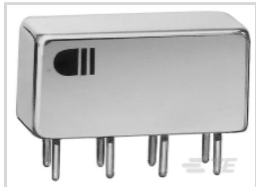
Relay & Contactor Type: **General Purpose Signal Relay**Current Type: **DC**Coil Magnetic System: **Non-Polarized, Monostable**Contact Arrangement: **2 Form C DPDT-CO**Contact Current Rating: **2 A**[All DPDT Signal Relay: Electrically-Held, With Coil Suppression \(46\)](#)
