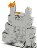
14 mm PLC basic terminal block with screw connection, without relay or solid-state relay, for mounting on DIN rail NS 35/7,5, 2 changeover contacts, input voltage 230 V AC/DC
