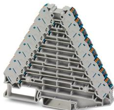
Marshalling panel, nom. voltage: 250 V, nominal current: 8 A, connection method: Push-in connection, 1st, 2nd, 3rd, 4th, 5th, 6th, 7th and 8th level, Rated cross section: 1.5 mm<sup>2</sup>, cross section: 0.14 mm<sup>2</sup> - 2.5 mm<sup>2</sup>, mounting: NS 35/7,5, NS 35/15, color: gray, color of connection elements: blue
