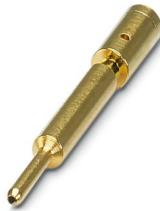
Crimp contact, Pin, turned, Single contact, contact diameter: 1 mm, crimp range: 0.5 mm<sup>2</sup> ... 1 mm<sup>2</sup>
