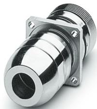
M23, Front panel feed-through, series: RC, straight, shielded: yes, Screw locking mechanism, No. of pos.: 8+1, Direction of rotation: Standard, contact connection type: Socket, Crimp connection, Flat gasket, 4x Ø 3.2, Panel thickness min.: 3 mm, Panel thickness max.: 7 mm, cable diameter range: 7.5 mm ... 9.5 mm, coding: N, Alternative product in accordance with RoHS II without Exemption 6c (Pb < 0.1 %) item no.: 1243124
