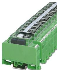
Relay module, with soldered-in miniature switching relay, contact (AgNi): medium to large loads, double A2 connection, 1 changeover contact, input voltage 230 V AC/DC
