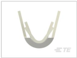
Splice Type: Pigtail Splice
