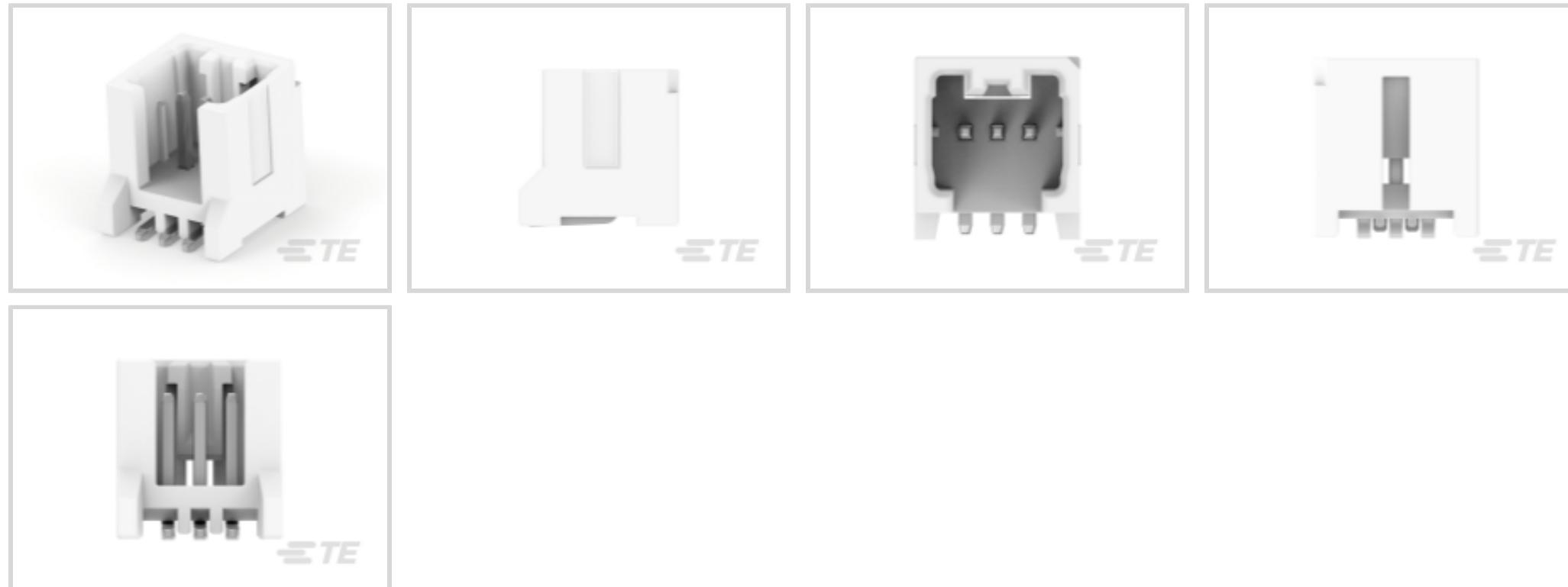
Connector Product Type: **Connector Assembly**Connector & Housing Type: **Plug**Connector System: **Wire-to-Board**Number of Positions: **3**Centerline (Pitch): **1.2 mm [.047 in]**
