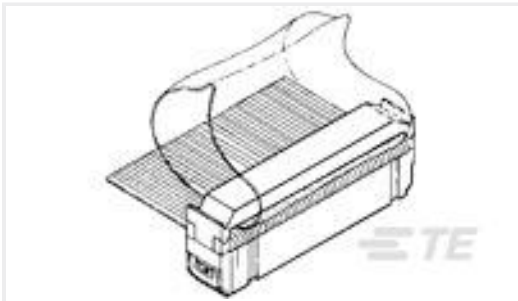
TE Part #5088450-8 PULL LOOP, CUT LENGTH 1.58 IN
