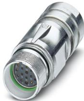
M23, Coupler connector, series: CA, straight, shielded: yes, for standard and SPEEDCON interlock, No. of pos.: 16+2+FE, Direction of rotation: Standard, contact connection type: Socket, Crimp connection, cable diameter range: 6 mm ... 10 mm, coding: N, Alternative product in accordance with RoHS II without Exemption 6c (Pb < 0.1 %) item no.: 1245043
