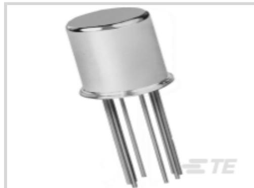
Relay & Contactor Type: **General Purpose Signal Relay**Current Type: **DC**Coil Magnetic System: **Non-Polarized, Monostable**Contact Arrangement: **1 Form C SPDT-CO**Contact Current Rating: **1 A**
