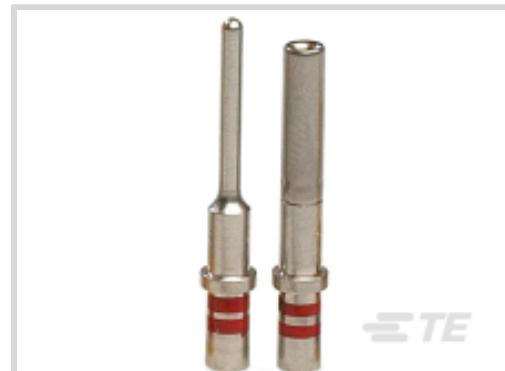
Contact Type: **Pin**Operating Voltage: **115 VDC**Contact Retention Within Housing: **With**Contact Retention Type Within Housing: **Spring****Features****Contact Features**
