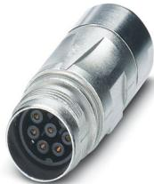
Coupler connector, straight, for standard and SPEEDCON interlock, M17, number of positions: 5+3+PE, contact connection type: Socket, shielded: yes, degree of protection: IP67, cable diameter range: 5 mm ... 9.2 mm, number of positions: 9, connection method: Crimp connection, series: ST, Alternative product in accordance with RoHS II without Exemption 6c (Pb < 0.1 %) item no.: 1243308
