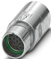
M23, Coupler connector, series: M23 PRO, straight, shielded: yes, for standard and ONECLICK fast locking system, No. of pos.: 17, Direction of rotation: Standard, contact connection type: Socket, Crimp connection, cable diameter range: 4 mm ... 8.5 mm, coding: N, Item is lead-free in accordance with RoHS II without Exemption 6c (Pb < 0.1 %)
